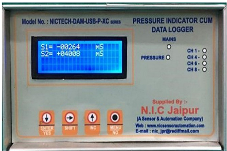
FIGURE 6: Digitizer cum data logger displaying microstrain values
