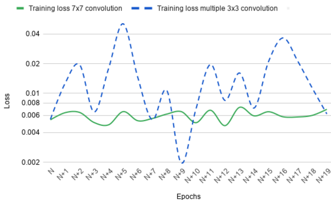
Figure 2. Training loss of two different type convolution networks. The training loss was extracted from a 20 epoch window while training. N depicts the start of the window and the loss was plotted for each epoch. Training loss of convolution network with two different kernel sizes ( 3 \times 3 and 7 \times 7 ) are plotted.
