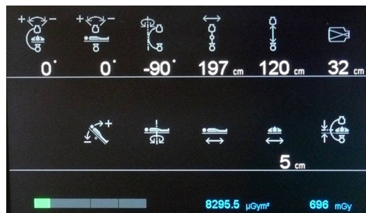
Fig. 3 Display of geometrical and dose parameters in the interventional room with cumulative KAP and K_{ar}
