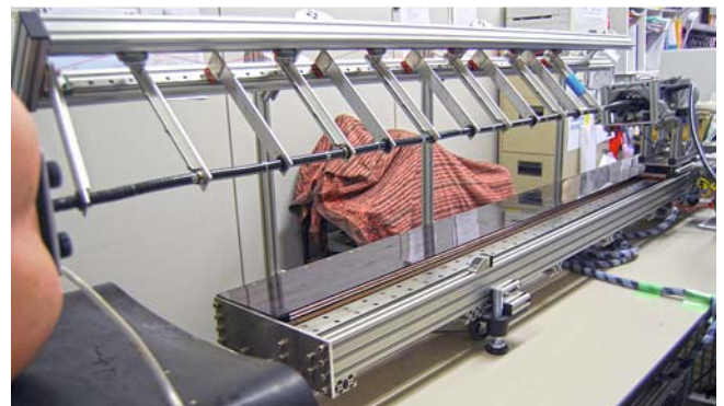
► Fig. 2 The slave unit of Endoscopic Operation Robot (EOR) ver. 3. to which the colonoscope (Olympus PCF-240; Tokyo, Japan) is attached.
