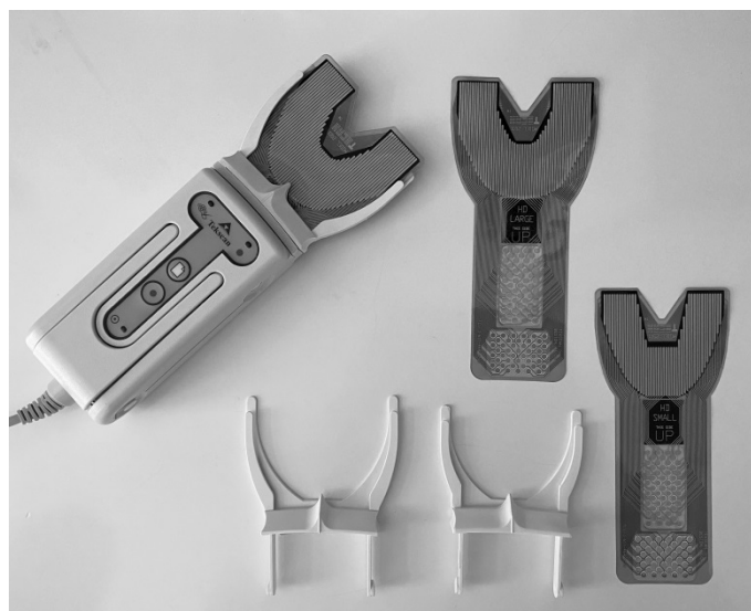
Figure 1. T-scan III panel (handle) that enables registration and a para-occlusal holder equipped with the sensor—100-micron-thick articulating foil.
