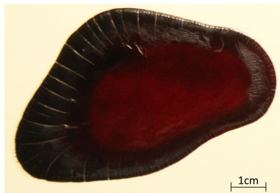
Figure 12. Pool drying at 22.5 °C on a white tile.
