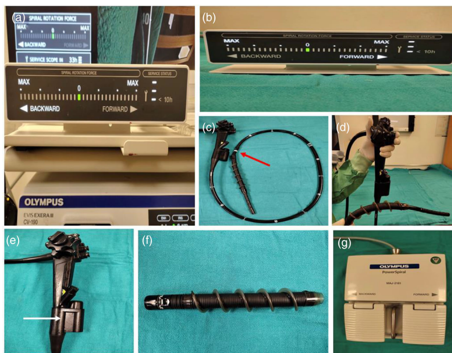
FIGURE 2 (a) Novel motorized power spiral enteroscopy system with power spiral (PSF-1; Olympus Medical Systems, Tokyo, Japan). (b) A visual force gauge used to monitor the direction and force applied to the tissue by the spiral rotation of the enteroscope. (c–e) Reusable power spiral enteroscope with an integrated electric motor (white arrow); 1680 mm working length, 11.3 mm outer diameter (insertion portion), with 140° forward view, 180° up and down bending, and 160° left-right movement, 3.2 mm accessory channel with dedicated separate irrigation channel. (f) Short disposable overtube with atraumatic soft spiral fins (240 mm length, 31.1 mm outer diameter of the spiral fins) attached to the rotation coupler (red arrow) located 40 cm proximal to the endoscope's tip. (g) Footswitch to control the direction and speed of motorized rotation of the spiral section
