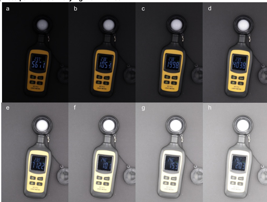
Supplementary Fig. 16. Black photo panel as a function of illuminance measured using a lux meter at consistent camera setting: (a) 567 lux, (b) 1054 lux, (c) 1998 lux, (d) 4038 lux, (e) 7122 lux, (f) 10100 lux, (g) 15300 lux, and (h) 20300 lux. The camera shutter speed is at 1/25 s and f number = f/5.6.
