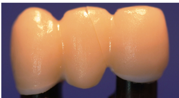
Figure 5 Fracture made in group 4 through the connector and the pontic.
