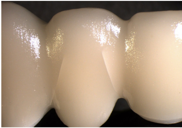
Figure 4 Visible radial cohesive veneer fracture in groups 2, 3, and 6.
