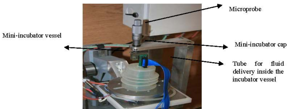
Figure 8. Mini-incubator for monitoring of cell cultures.
