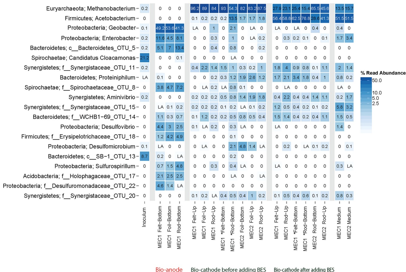
FIG 7 Relative abundances of the 20 most abundant 16S rRNA gene sequences in the bioanodes, biocathodes before and after adding 2-bromoethanesulfonate (BES), medium at the end of the experiment, and inoculum. LA refers to abundances of <0.1%. *, electrodes that were placed in MEC1 after removing bioanodes.
