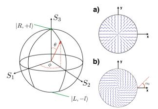
**Figure 1** | Left: Hybrid-Poincaré sphere (HPS) representation for a vector vortex beam state of polarization. Right: q-plate geometries for the case q=1 and a)  $\alpha_0=0$ , b)  $\alpha_0=\frac{\pi}{4}$ . Blue lines represent local optic axis orientation.
