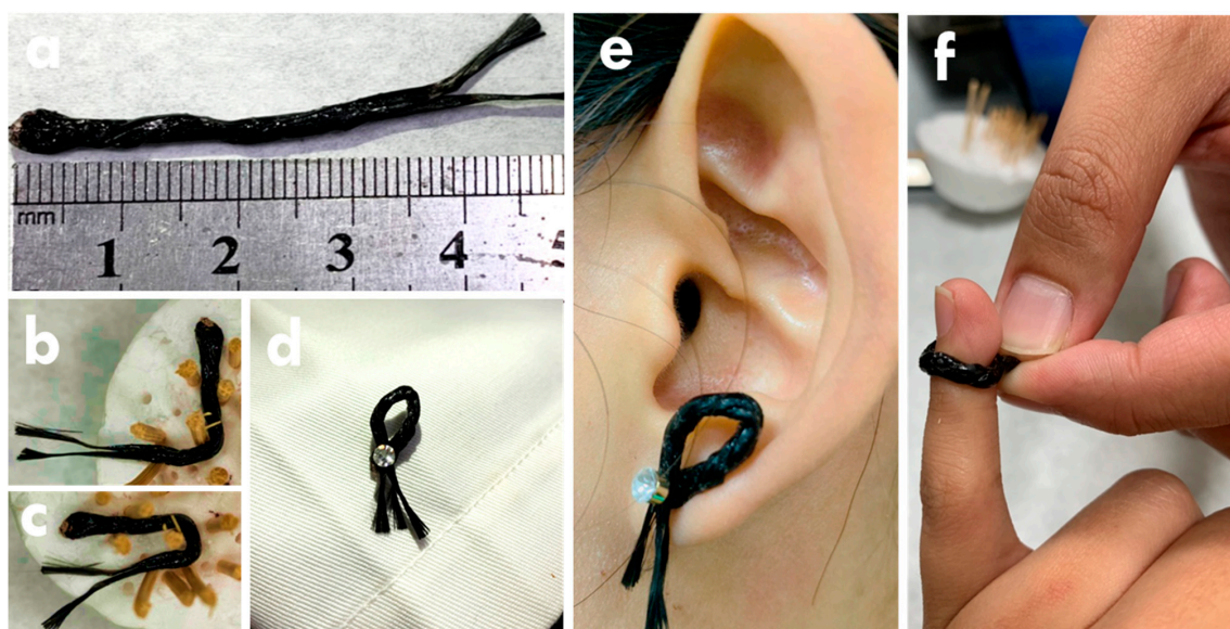
Figure 8. The photos for the FSC (a) without bending, (b) bended in 90°, (c) bended in 180°, bended in the circle shape and (d) attached in cloth, (e) wore as the earring, and (f) wore as the ring.
