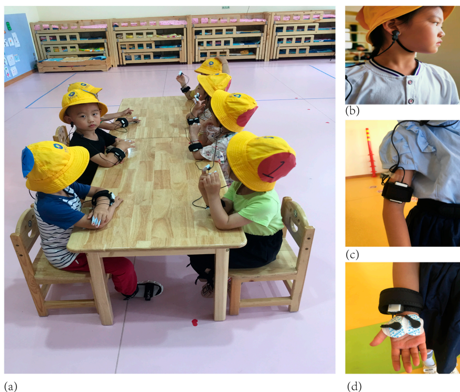
Figure 1. (a) Experimental scene; (b,c) Data collector and receiver for heart rate variability (HRV); (d) Data collector and receiver for electrodermal activity (EDA).
