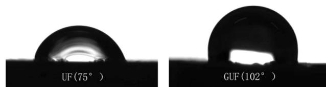
Figure 1. Water contact angles of UF and MMU–G.
