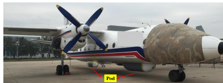
Figure 1. The installation layout of SAR antennas (in the pod below the belly).
