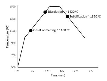
**Figure 5.** Temperature vs. time of the CoCrCu + Ni samples heated and imaged from 1000 °C to 1500 °C and back down to 1000 °C.
