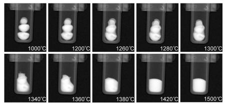
**Figure 7.** Radiographs taken at increasing temperatures of the CoCrCu + Ni buttons inside the alumina crucible in the HOT-A vacuum furnace. A full movie-like sequence of radiographs can be found in the Supplementary Materials.
