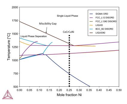
**Figure 9.** Calculated isopleth of the CoCrCuNi<sub>*x*</sub> system using Thermo-Calc software. Legend descriptions: SIGMA ORD = ordered  $\sigma$  phase, FCC<sub>L12</sub> DISORD = disordered FCC phases, BCC<sub>B2</sub> DISORD = disordered BCC phases.
