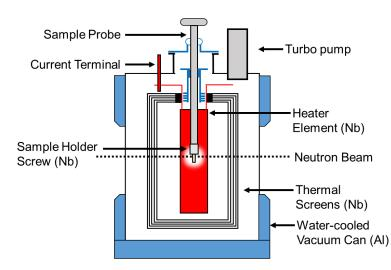
**Figure 3.** Top loading neutron furnace layout and description of furnace elements. More information pertaining to this furnace can be found in Ref. [24].
