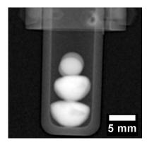
**Figure 4.** Radiograph of the four buttons stacked inside an alumina crucible such that the heterogeneous CoCrCu are placed on the bottom while the spheres of Ni are placed at the top (the Ni buttons are oriented in the direction of the beam such that they overlap). The darker regions present randomly in the bottom two buttons are the Cu-rich phase that separated in the liquid during arc-melting of the CoCrCu buttons.
