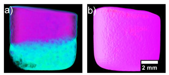
**Figure 8.** (a) Reconstructed computed tomography (CT) of the solidified heterogenous CoCrCu alloy recreated from Ref. [23] with permission from the authors. (b) Reconstructed CT of the solidified CoCrCuNi alloy.
