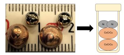
**Figure 1.** Photograph of the arc-melted CoCrCu buttons next to the remelted Ni buttons prior to the neutron imaging and melting.
