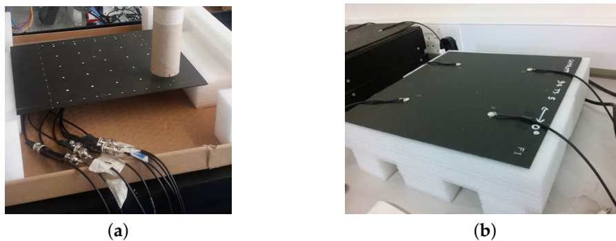
Figure 1. Composite panel subjected to the experimental tests. Top view (a); and bottom view with sensors (b).
