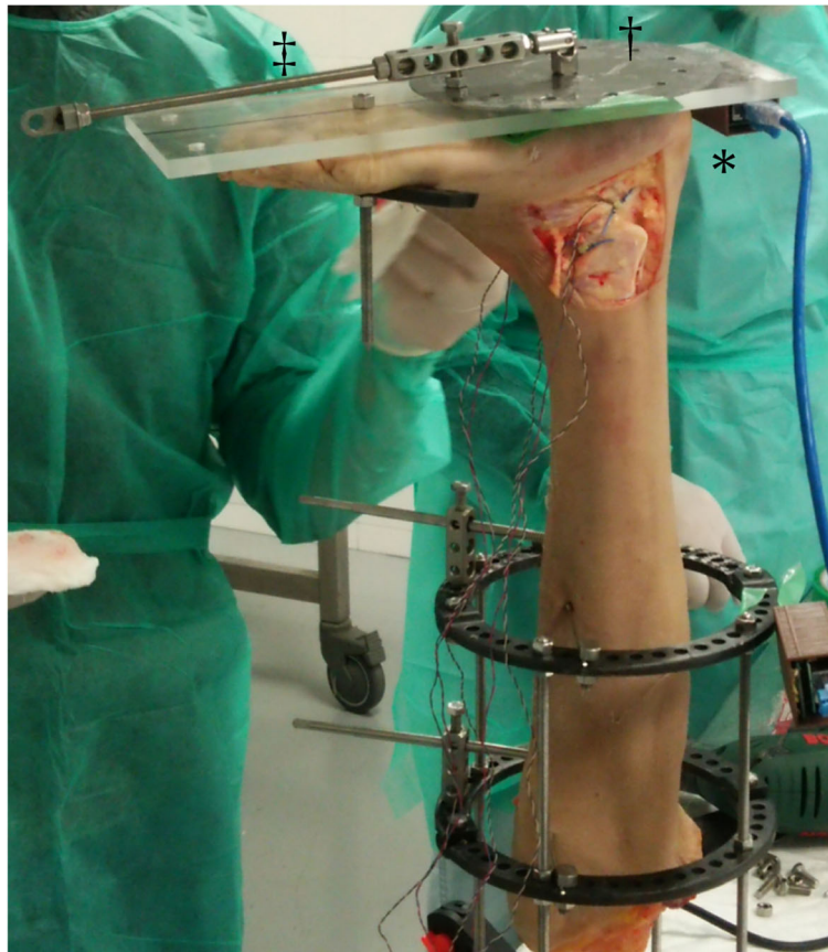
Fig. 3 Setup of the specimen. The lower limb is fixed vertically to the measurement desk using an Ilizarov ring-shaped external fixator, and a performance cube (*), clock (†) and an arm (‡) are affixed to an acrylic plate
