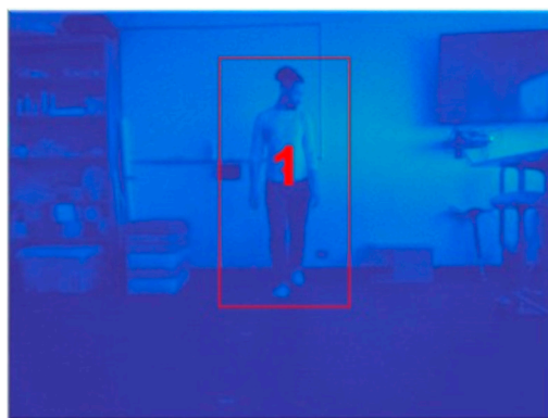
Figure 7. Smoothed centroid location with unique identifier and bounding box. Note: Figure 7 shows the Kalman filtered centroid location, where the centroid location is indicated by the unique numerical identifier (i.e., “1”). A bounding box also appears around the object of interest.
