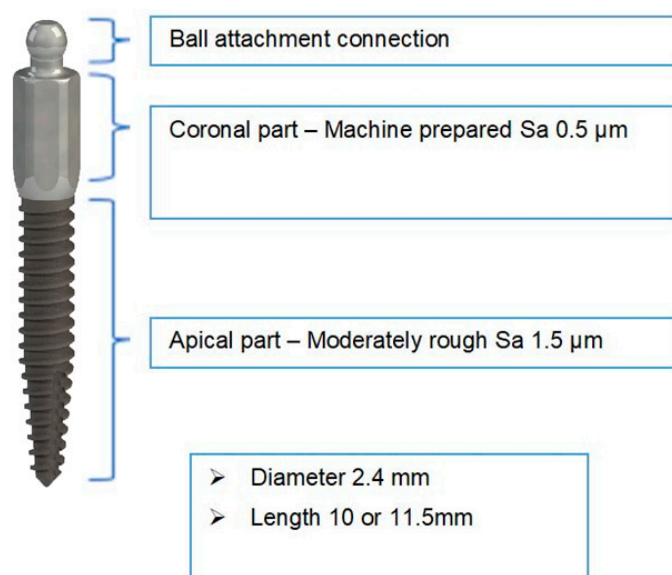
Figure 1. ILZ prototype mini-implant Southern Impl., Inc., Irene, South Africa.
