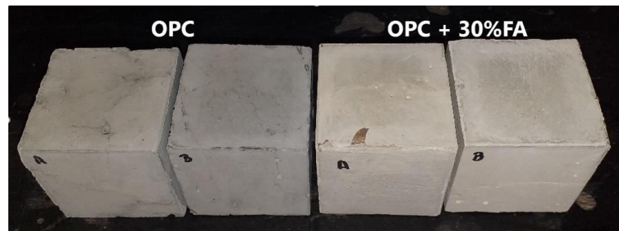
Figure 2. Five cm cubic specimens bearing 100%OPC and 70%OPC + 30%FA.
