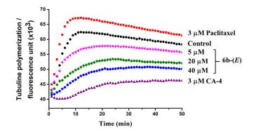
**Figure 6.** Effects of **6b-(E)** on tubulin polymerization in vitro. Tubulin (10 mg/mL) was incubated with **6g-(E)** (5, 20 and 40  $\mu$ M) for 50 min at 37 °C. Paclitaxel (3  $\mu$ M) and CA-4 (3  $\mu$ M) were used as positive controls. The fluorescence intensity was monitored every minute for characterization of tubulin polymerization at a 360 nm excitation wavelength and 460 nm emission wavelength.
