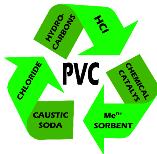
Figure 6. Main directions of substance recovery as a result of feedstock recycling of PVC.
