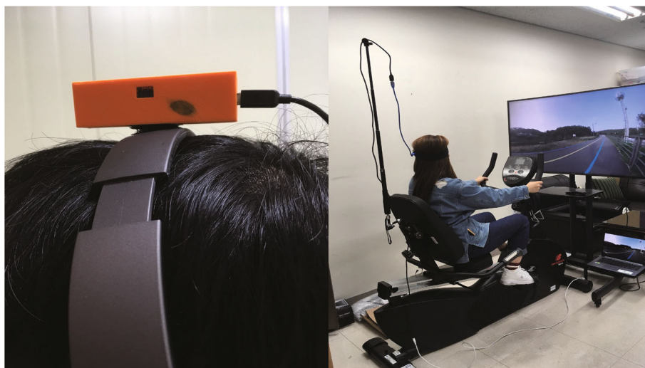
Fig. 4 MPU6050 sensor-based head tracking system and experimental setup
