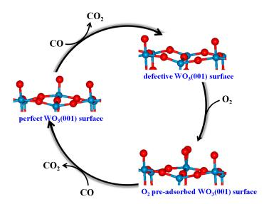
**Figure 6.** Schematic representation of a possible full sensing cycle of the WO<sub>3</sub>(001) surface as a CO sensor.
