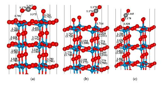
**Figure 4.** Oxidation product for CO reacting with (a) the  $O_t$  atom on perfect  $WO_3(001)$  surface; (b) the O atom belongs to the  $O_2^-$  species and (c) the  $O_t$  atom on defective  $WO_3(001)$  surface modified by the pre-adsorbed  $O_2$  molecule.
