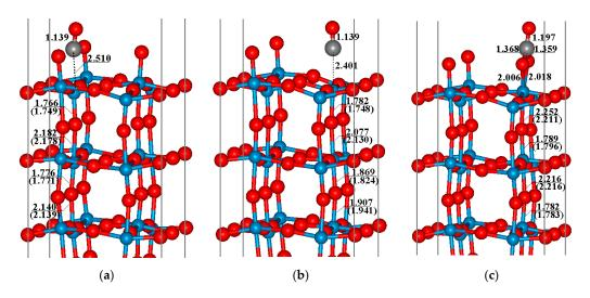
**Figure 3.** Adsorption structures of CO on (a) perfect WO<sub>3</sub>(001) surface; (b) defective WO<sub>3</sub>(001) surface, and (c) defective WO<sub>3</sub>(001) surface modified by the pre-adsorbed O<sub>2</sub> molecule. The data in the parenthesis is corresponding to the value before CO adsorption.
