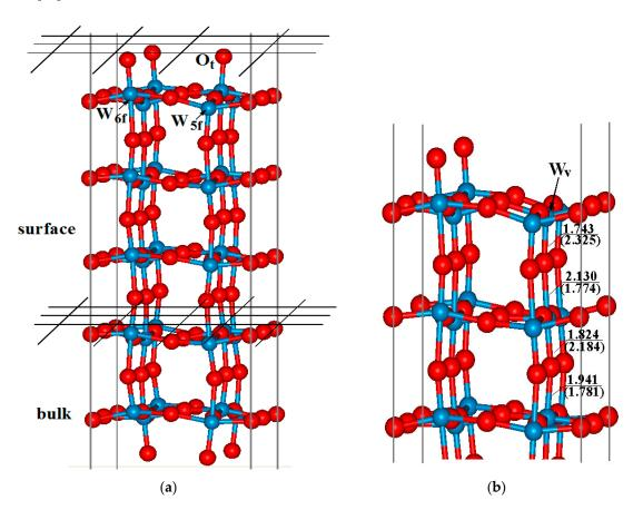
**Figure 1.** Configuration of (**a**) five-layer perfect WO<sub>3</sub>(001) surface and (**b**) defective WO<sub>3</sub>(001) surface with half of the top oxygen atoms missing. The blue and red balls stand for tungsten and oxygen atoms, respectively.
