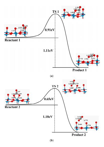
**Figure 7.** Minimum energy paths (MEP) for CO oxidation on (a) the perfect and (b) the  $O_2$  pre-adsorbed WO<sub>3</sub>(001) surface. The configurations of the top layer and some bond distances (Å) of the initial and final states, as well as the transition state (TS) are also shown in the figures.
