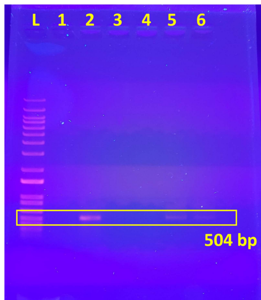
Fig. 6. Electrophoretic analysis of bacterial genomic DNA extracted from the clinical sample and amplified with P. aeruginosa primer set using the proposed thermal management system. Lane L, 1Kb DNA marker, Lane 1 (Negative control), 2 (Positive control), RPA amplified amplicon with oprL primer set (504 bp) performed in microreactor chamber, Lane 3, 4 no DNA template (Negative control) with each primer set, lane 5, 6 contain DNA template (Positive control) PCR-generated amplicon with oprL (504 bp) primer set performed in a thermal cycler.
