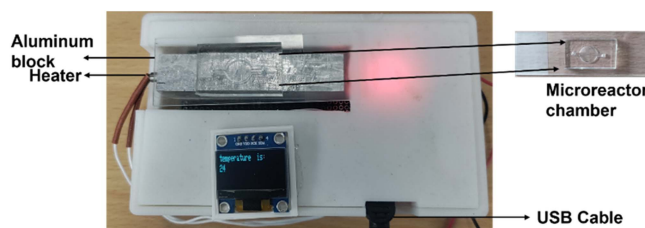
Fig. 2. 3D package of the thermal management device with a microreactor placed on it.
