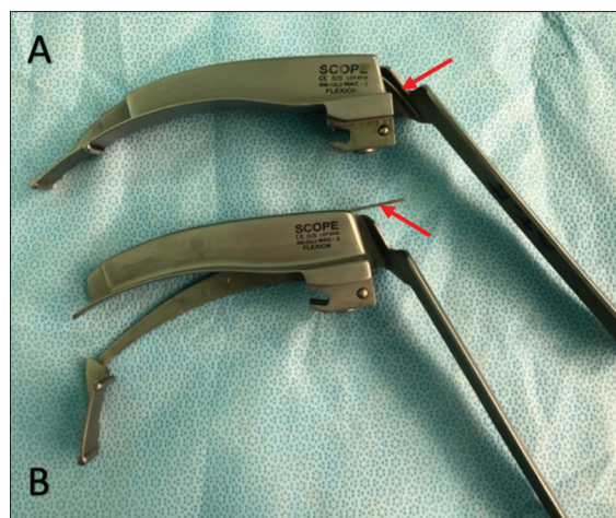
Figure 1: Failure of hinged tip mechanism due to slipping of loaded spring. Spring labelled with pointer. A - Normal laryngoscope; B - Failed laryngoscope
