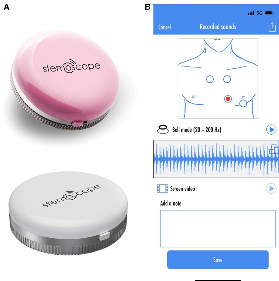
Fig. 4 A Stemoscope. B Stemoscope app to record heart sounds. The red dot on the screen is tapped to start recording sounds. Then, the investigators can play the recorded sounds. The app provides several options to share recorded sounds, such as via Twitter, Facebook, and WeChat
