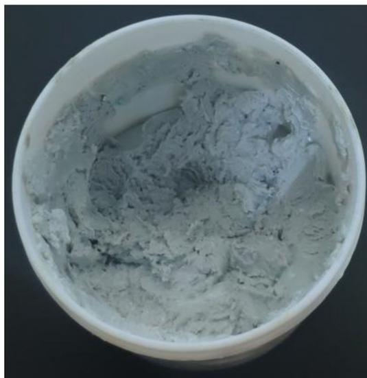
**Figure 1.** The physical appearance of plastic steel soil.
