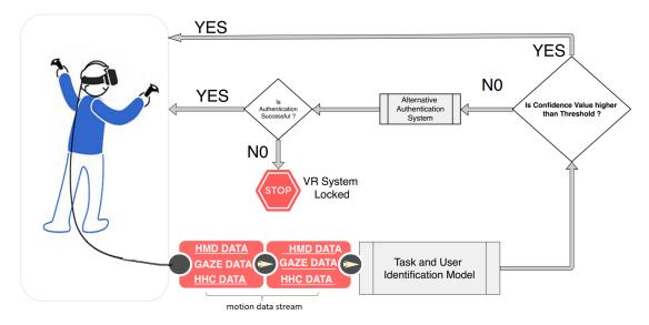
**Figure 2.** A diagram of the BioMove biometric identification process. As the user performs activities within the virtual reality environment, the motion data stream is passed to the Identification Model which determines the task and the user performing the task. A confidence value from the model is used to determine if the user is an authorized user. If the user is not an authorized user, the VR session, for example, can be stopped.
