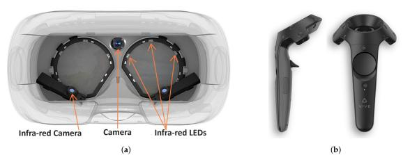
**Figure 4.** (**a**) The HMD upgraded for Gaze tracking: Interior view of a HMD device fitted with eye tracking hardware. (**b**) VR Hand-Held Controller (HHC) used in our study by participants to interact with VR objects with 6-DOF.
