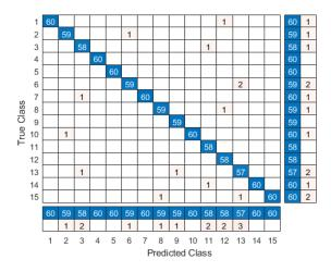
**Figure 9.** kNN Classifier Confusion Matrix: A confusion matrix summarizes the performance of a classification algorithm. It gives a better idea of what your classification model is getting right and what types of errors it is making. Classification accuracy alone can be misleading because we have more than two classes in our dataset.
