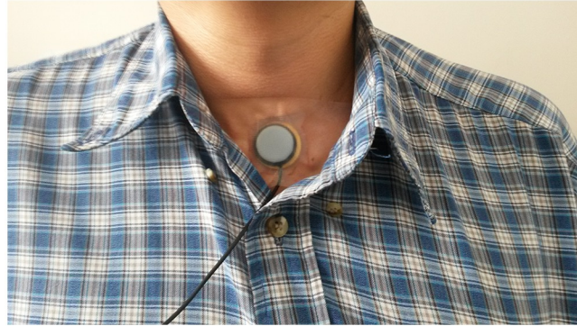
Fig 1. Piezoelectric sensor. Shown here is the vibrometer, as it would be worn by a participant.
