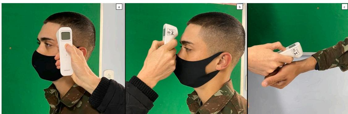
Fig. 3. Setup of thermal data acquisition in different body regions: temple (a), forehead (b), wrist (c)
