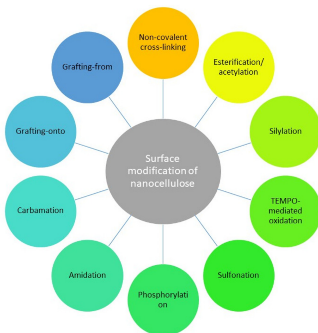
Figure 4. Surface modification methods of nanocellulose (summarized from Ghasemlou et al. [51]).
