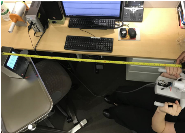
FIGURE 2. 1 m from airflow head to device port.
