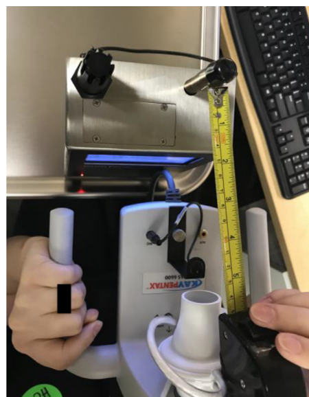
FIGURE 1. 15 cm from airflow head to device port (port is capped in this image but was uncapped for data collection).
