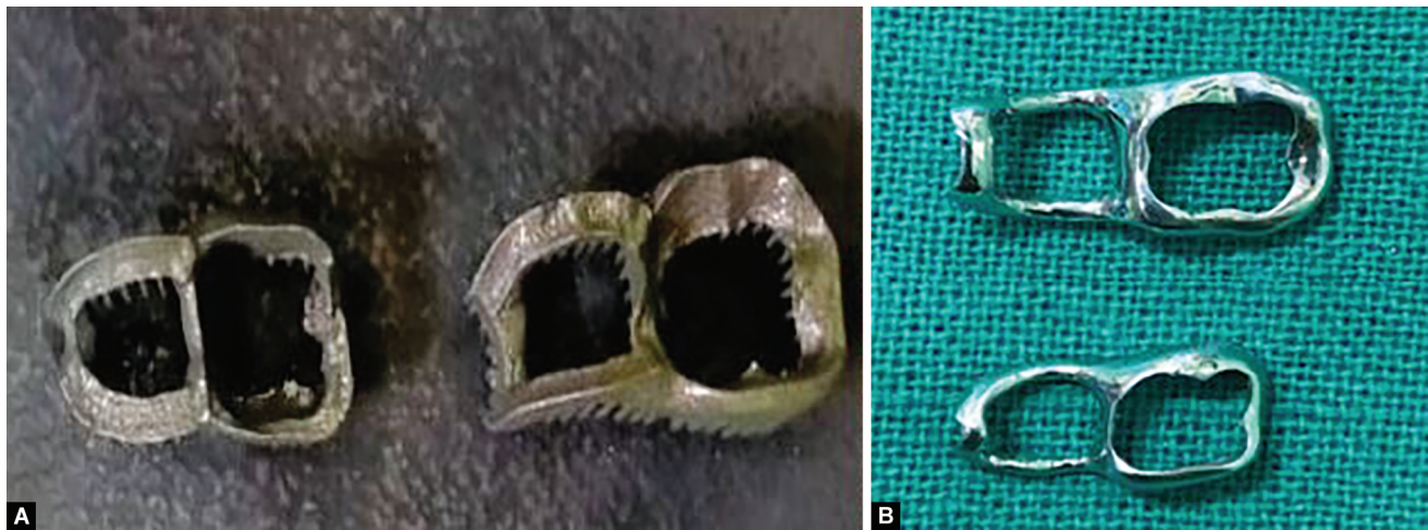
Figs 3A and B: (A) Prefinal outlook of 3D printed cobalt- chromium base alloy metal-based band and loop space maintainer; (B) Final outlook of 3D printed Co-Cr base alloy metal-based band and loop space maintainer
