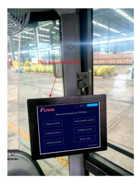
Figure 10. Data acquisition device installed in the cab of the FW50GL wheel loader.
