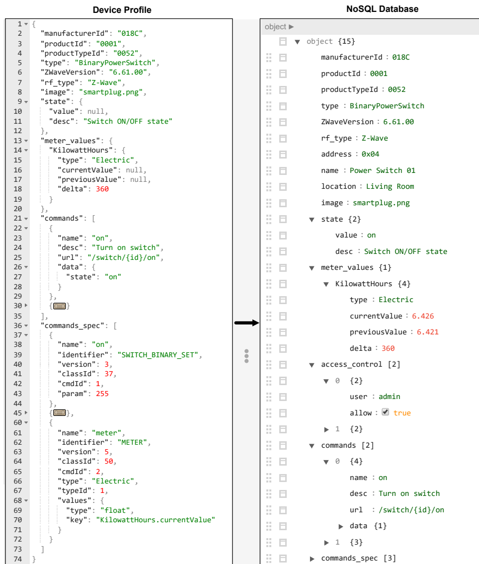
Figure 4. All information of a device is stored in the NoSQL database as a virtual device.
