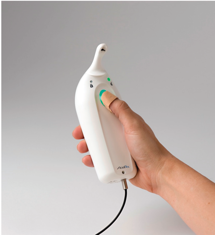
FIGURE 1. Sufentanil sublingual tablet system with RFID patient thumb tag and security tether attached to the bottom of the controller.
