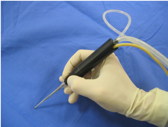
Figure 1 Penstyle micro handpiece with his micro sonotrode: length 192 mm, weight 60 gr, end diameter of the top 1.45 mm, used as a pen.
