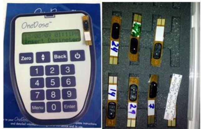
Fig. 1 The OneDose system with the detector (Left), and close-up of the detector (Right).
