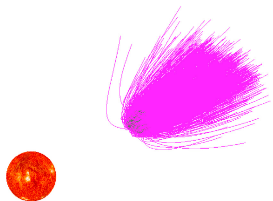
Figure 4. Trajectories of dust around Benu. The trajectories are plotted relative to the inertial space. Dust grains are ejected from the asteroid surface. 2000 dust grains are generated. To see the influence of the solar radiation on the motion of dust grains, the Sun is plotted in the solar direction.
