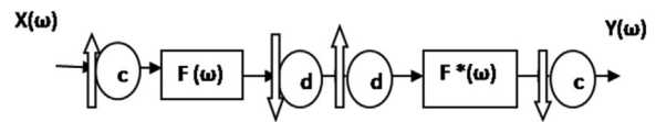
(b) The system represented in Fig. (a) is made up of linear combinations of the systems shown above
