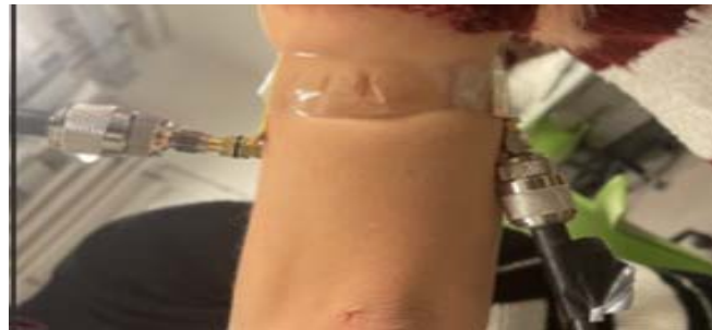
Figure 11. The fabricated pair of antennas are placed on a real human arm of radius 45 mm to examine the transmission coefficient.
