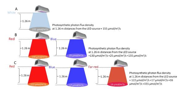
**Figure 2.** The photosynthetic photon flux densities (PPFD) of the Heliospectra<sup>TM</sup> grow lights measured using a LaserCheck optical power meter, at different distances from the light-emitting diode (LED) source, for all tents.
