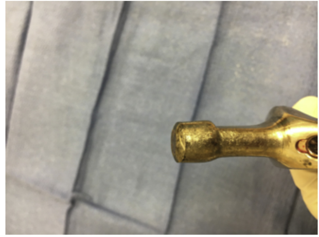
Figure 6. Intra-operative trunnionosis: intra-operative findings of trunnion corrosion and scratching after femoral stem explant (DePuy Corail).
