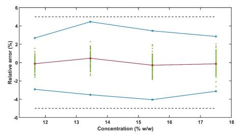
Figure 13. Accuracy profile with the dashed black lines indicating  $\pm 5\%$  limits, the blue lines with circles are the  $\beta$ -expectation tolerance limits, green points are the relative bias for every measurement and the red line with circles is the method mean relative bias.
