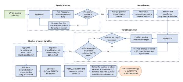
**Figure 4.** Methodology to build predictive model using UV-Vis spectra. WL= wavelength, PCA = principal component analysis,  $R_{cv}^2$  = coefficient of determination, RMSECV = root mean square error, CV = cross-validation, LV= latent variables.
