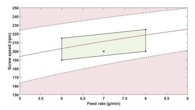
**Figure 14.** Contour profiler showing the influence of the interaction of screw speed and feed rate on the predicted PRX amount using the PLS model. The red line indicates the predicted PRX content of  $14.45\% \ w/w$ . The black cross marks the optimised extruder parameters. The black dashed lines indicate the upper and lower limits defined respectively 14.75 and  $14.15\% \ w/w$  of PRX.
