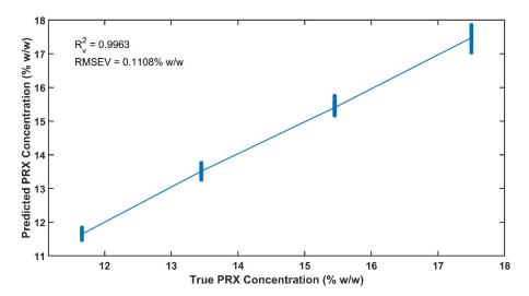
Figure 12. Linearity of the validation data set.
