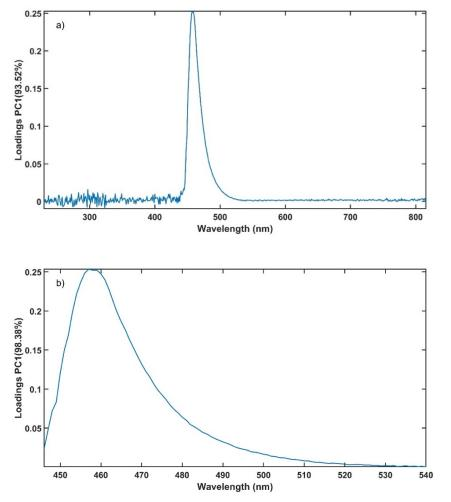
**Figure 10.** Loadings from a PCA of the calibration data set using (**a**) the entire wavelength range and (**b**) the selected range.
