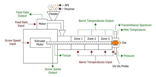
Figure 1. Schematic of the hot melt extrusion process.
