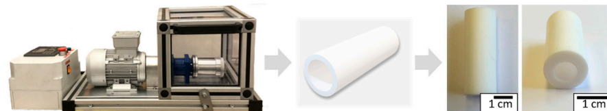
Figure 1. The equipment applied to produce samples by centrifugal slip casting with a photo of the manufactured specimen.
