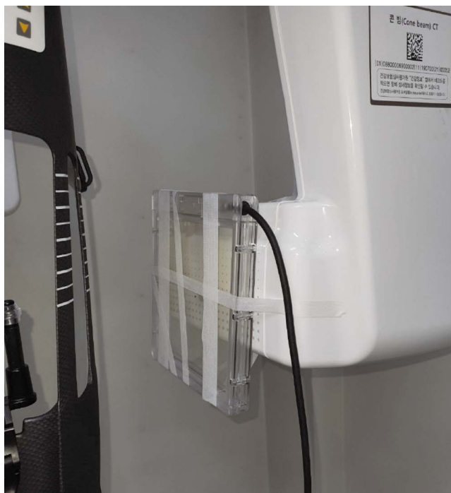
Fig. 1. A flat plane ionization chamber of a dose-area product meter is attached to the source side of the cone-beam computed tomography device.
