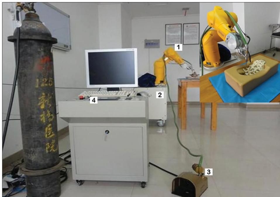
**Figure 1:** Spine robot system. (1) Robot arm, (2) Base of the robot arm, (3) Controller of the drill, (4) Console
