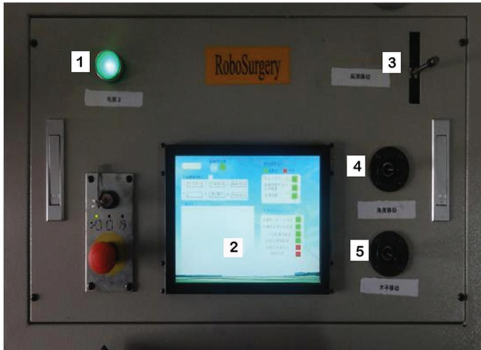
**Figure 2:** Operation interface of the console. (1) Power button (2) Touch screen operator interface (3) Operating lever longitudinal shift (4) Operating lever angular deflection (5) Operating lever horizontal shift
