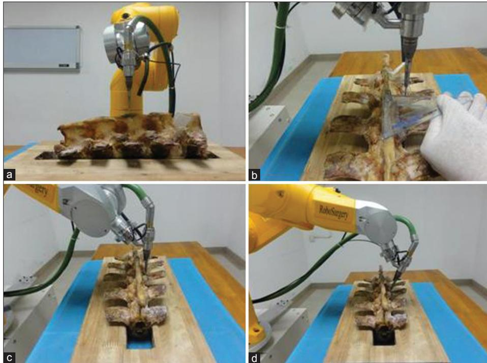
**Figure 4:** Percutaneous pedicle screws insertion. (a) Adjustment the pneumatic drill parallel to the upper vertebral body end plate, (b) Adjustment the distance between the tip of the drill and the posterior median line according to preoperative planned distance, (c) Longitudinal shift of the drill to the entry point on the bone surface, (d) Adjusting the entry angle of the drill according to preoperative planned angle
